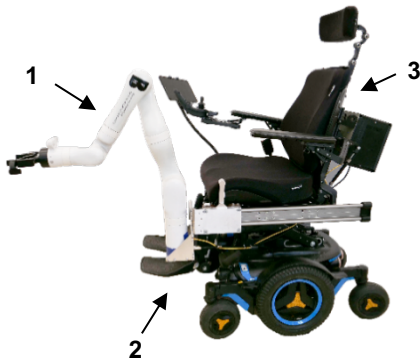
Fig. 1 Kinova Gen3 robot arm (1) mounted with the new construction (2) to a Permobil M3 wheelchair (3).
